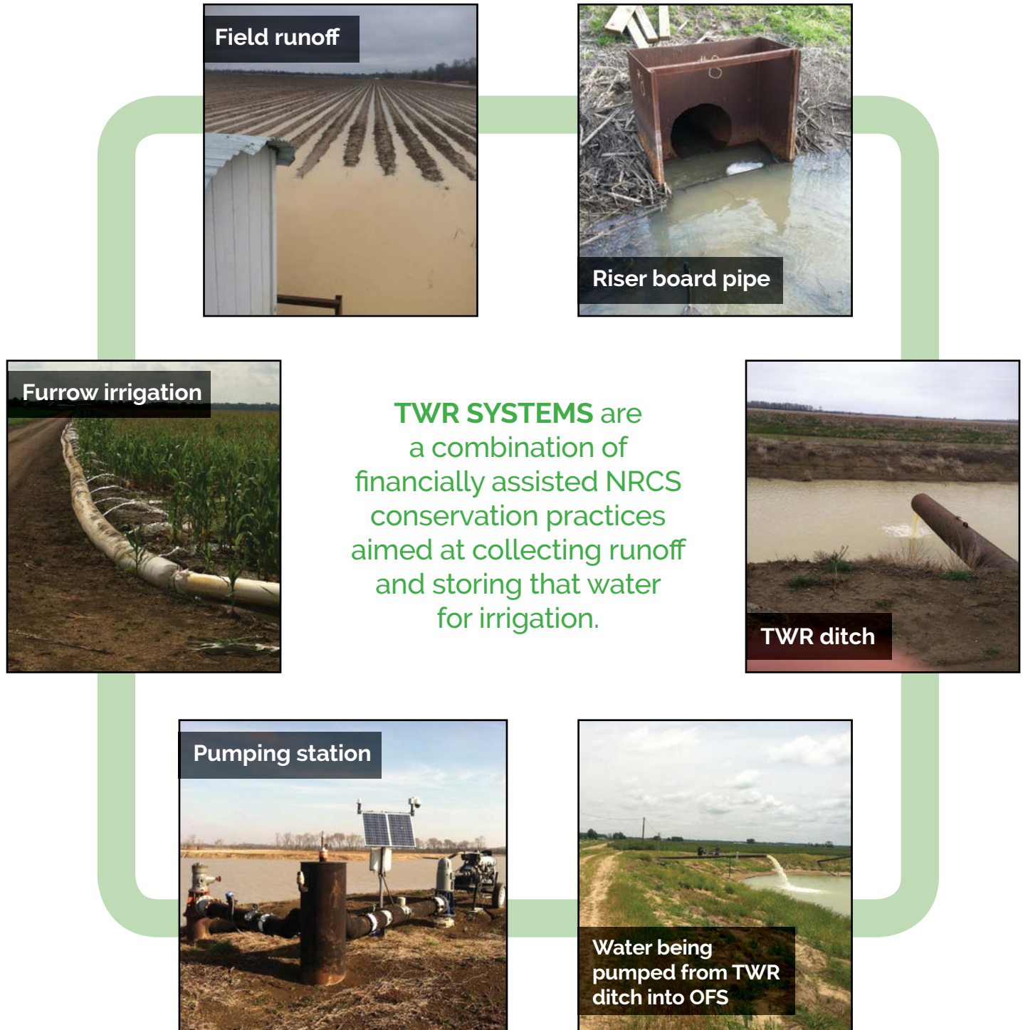
Figure 2. Water movement through a TWR system. Note that not all TWR systems have the same components. Some TWR systems are comprised of only a large TWR ditch and no OFS reservoir.
