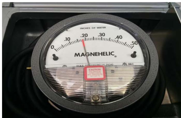
Figure 1. Hand-held Magnehelic static pressure gauge.
