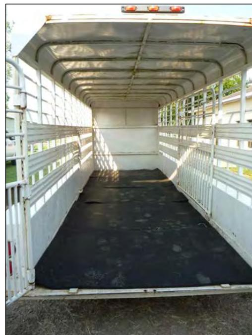
Figure 2. Rubber mats improve traction on trailer flooring.
