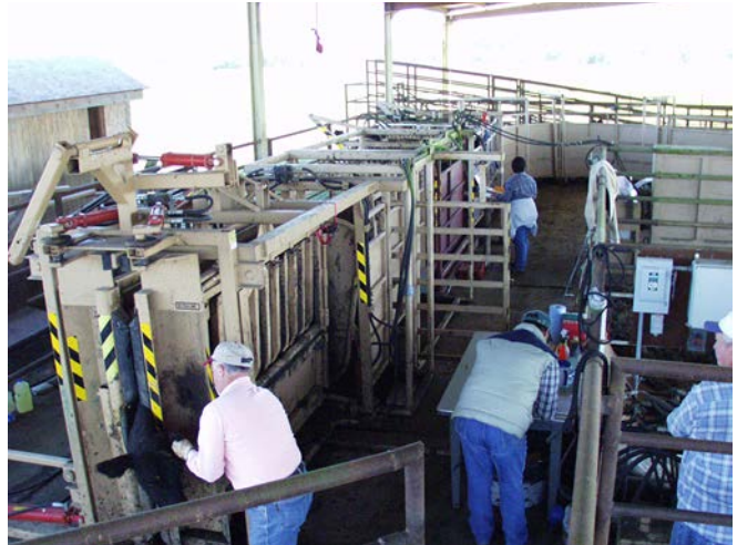
Figure 6. Slider (alley divider) extended outward between palpation cage and scale compartment.
