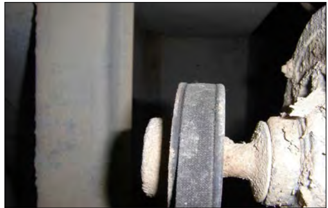
Figure 1. Fan belts should ride flush with or slightly above the top of the pulley.
