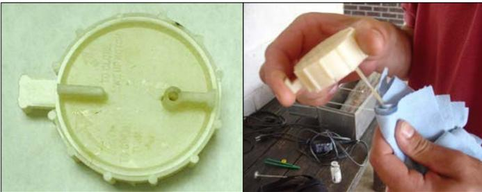
Figure 13. Straw cutting device.
