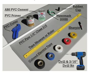
One set of 6-inch, 12-inch, 24-inch, and 36-inch sensors will require one 10-foot stick of ½-inch Class 315 PVC pipe. Select the correct PVC specifications to avoid frustrations later.
