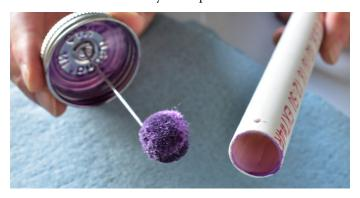
**Step 4:** After a few minutes of drying, thread the sensor wires from the bottom end of the PVC section to the top end until the sensor collar meets the bottom end. Bundle the extra wire.
