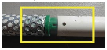
**Step 7:** Wrap a ring of black electrical tape so that the distance between the bottom of the tape and the middle of the attached sensor equals the intended sensor depth. After installation, the bottom edge of the black electrical tape should be flush with the ground.
