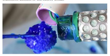
**Step 6:** While aligning the sensor weep slot with the drilled weep hole, push the sensor collar fully into the bottom end of the PVC section.
