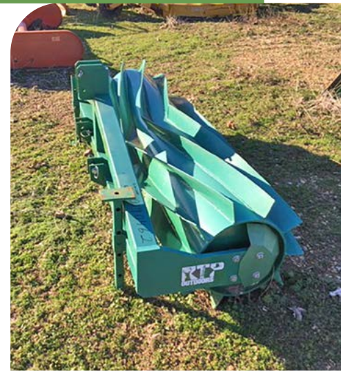
Figure 4. A roller-cripper uses weight to roll down plants, and the chevron pattern crimps the stems to terminate the plant. Water can be added to increase the weight and improve effectiveness.
