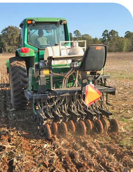
Figure 3. A seed drill allows planting at the proper depth and row spacing and maintains a uniform seeding rate per acre. Photo by Mark Shankle.
