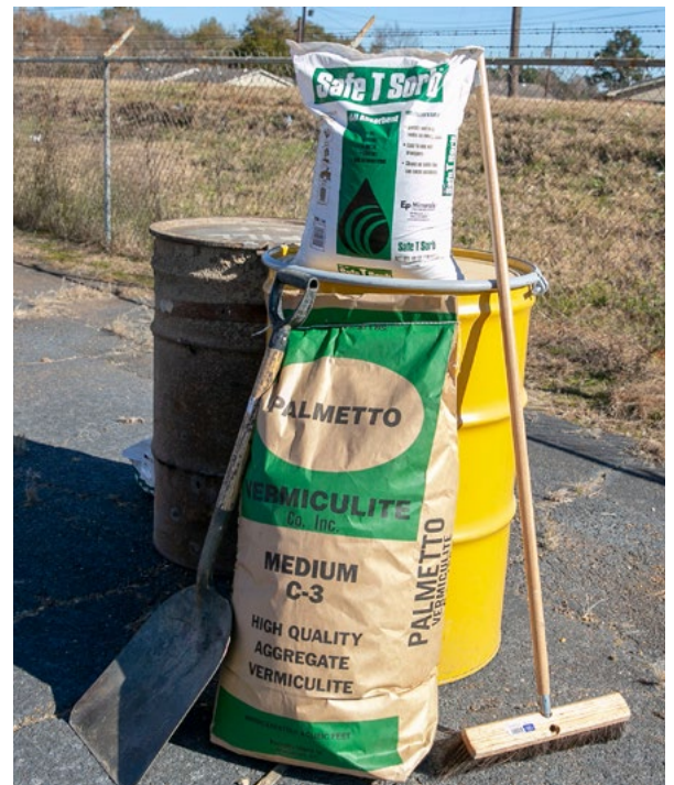
Figure 4. Absorbent materials, brooms, and shovels are good to have available during loading, unloading, and transport to help contain accidental spills.
