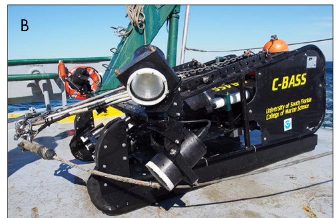
(A) An ROV, the VideoRay Pro 4, and (B) a towed camera, the Camera-Based Assessment Survey System (C-BASS), are used for direct visual counts.
