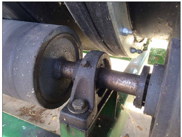
Figure 9. Grease fittings should be greased every quarter.
