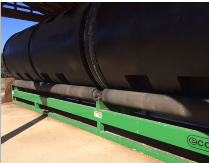
Figure 8. The drum turns on rollers located on each side of the unit.
