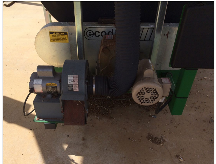
Figure 7. Blower pulls air through the unit to maintain correct oxygen level.
