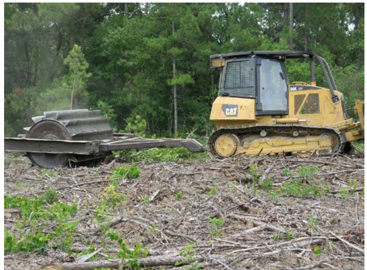
Figure 6. A drum chopper being pulled by a bulldozer. Photo by Andrew Ezell.
