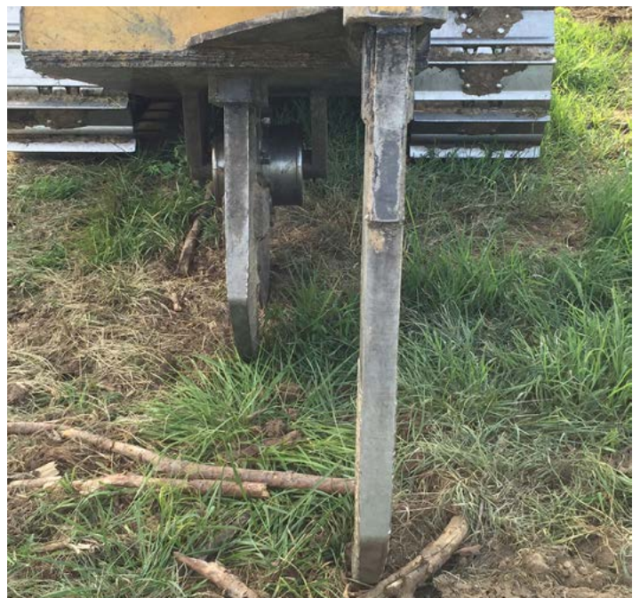
Figures 14 and 15. Offset double-shank subsoil system often used in cutovers. Note heavy-duty construction for increased shear-stress on tracts with increased roots and stumps.
