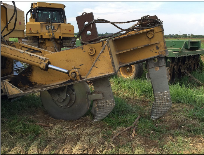
Figures 14 (above) and 15 (below). Offset double-shank subsoil system often used in cutovers. Note heavy-duty construction for increased shear-stress on tracts with increased roots and stumps. Photos by Brady Self and Andrew Ezell.
