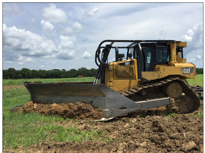
Figure 3. A V-blade attached to a bulldozer. Photo by Brady Self.
