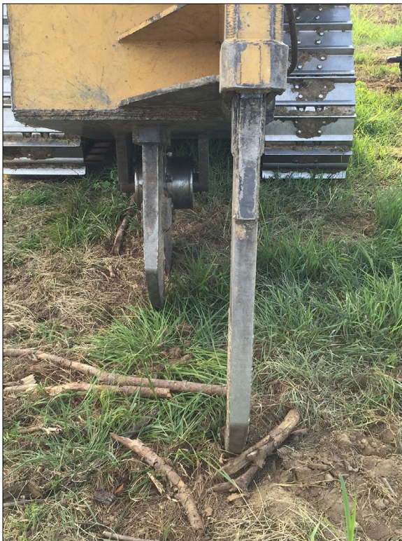
Figures 14 (above) and 15 (below). Offset double-shank subsoil system often used in cutovers. Note heavy-duty construction for increased shear-stress on tracts with increased roots and stumps. Photos by Brady Self and Andrew Ezell.
