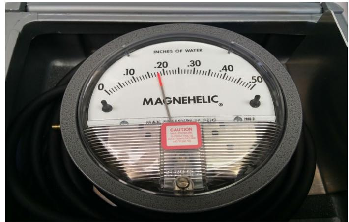
Figure 1. Hand-held Magnehelic static pressure gauge.
