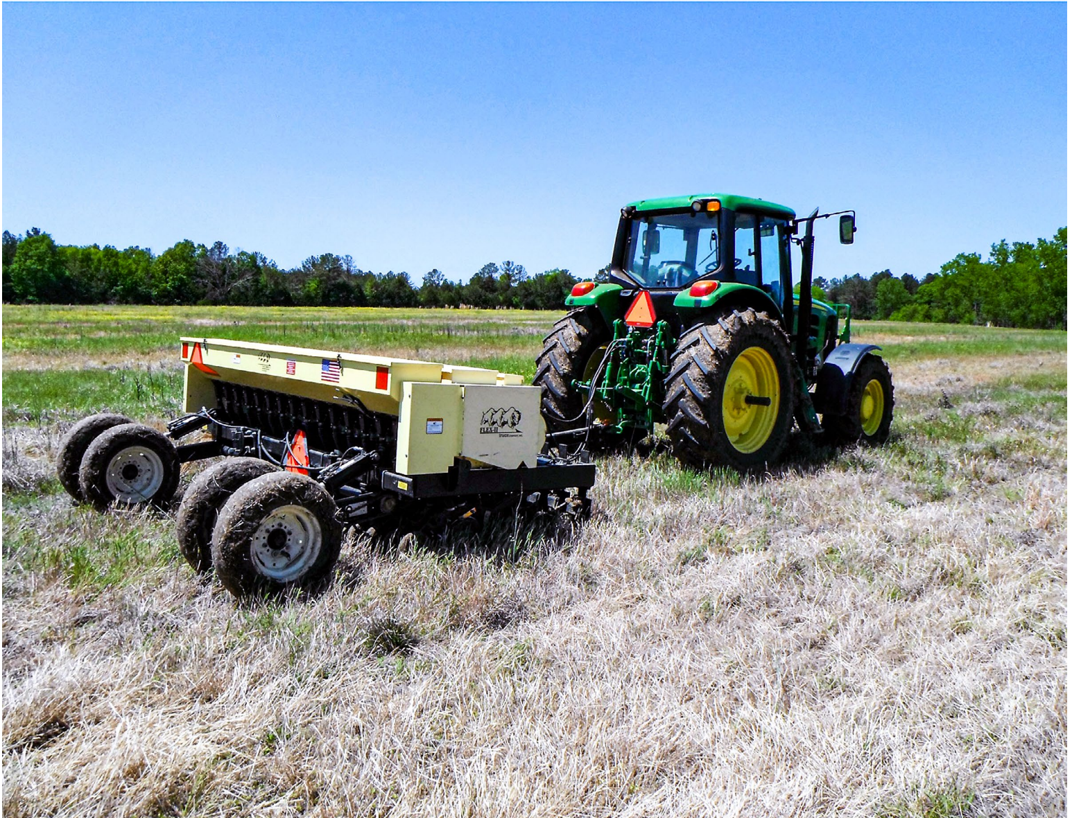
Figure 4. Native grass seed drills are designed to plant a variety of seeds, including fluffy or hairy NWSG seeds. This piece of equipment is highly recommended for establishing larger areas to native grasses, forbs, and legumes.
