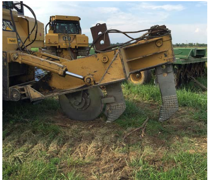
Figure 13. Double shank subsoiler used to prepare a former pasture for planting.
