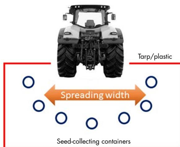
Figure 1. Configuration to determine the spreading pattern when calibrating a broadcast seeder.
