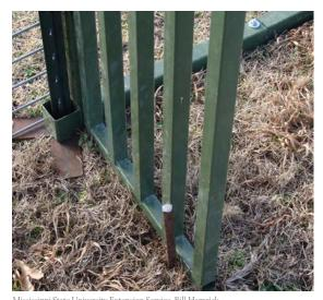
Placement of stakes behind each door panel on the inside of the trap.
