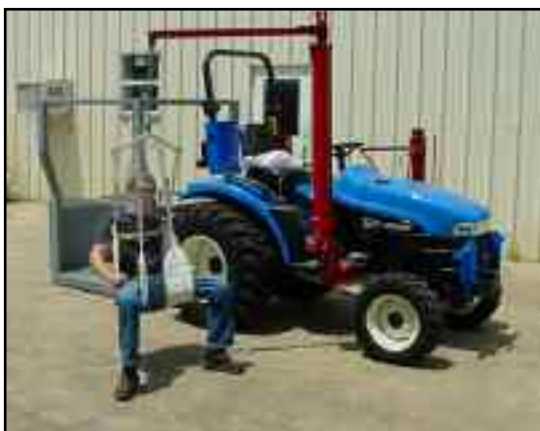
Pictured is a demonstration tractor equipped with a sling lift, a standing lift, hand controls, and a wheelchair platform.
