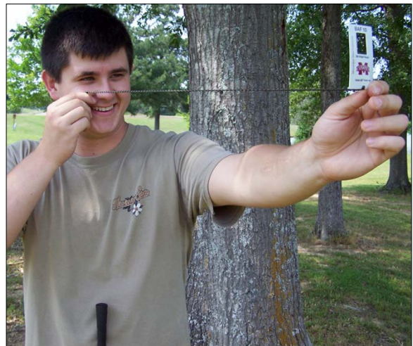
Figure 1. Using the MSU Basal Area Angle Gauge at 25 inches from eye. (Photo by Stephen Dicke)
