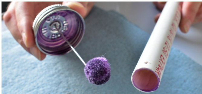
Figure 3.14. Apply PVC primer.
