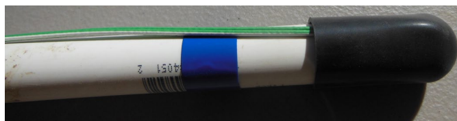
Figure 3.19. Add a rubber cap.
