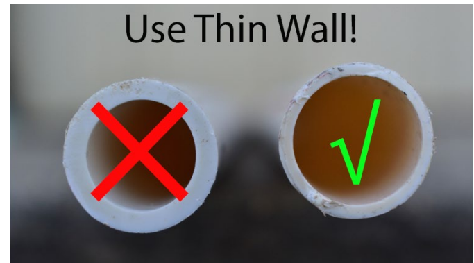
Figure 3.12. Use thin-walled PVC pipe.
