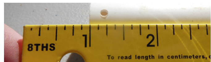
Figure 3.13. Drill the weep hole.
