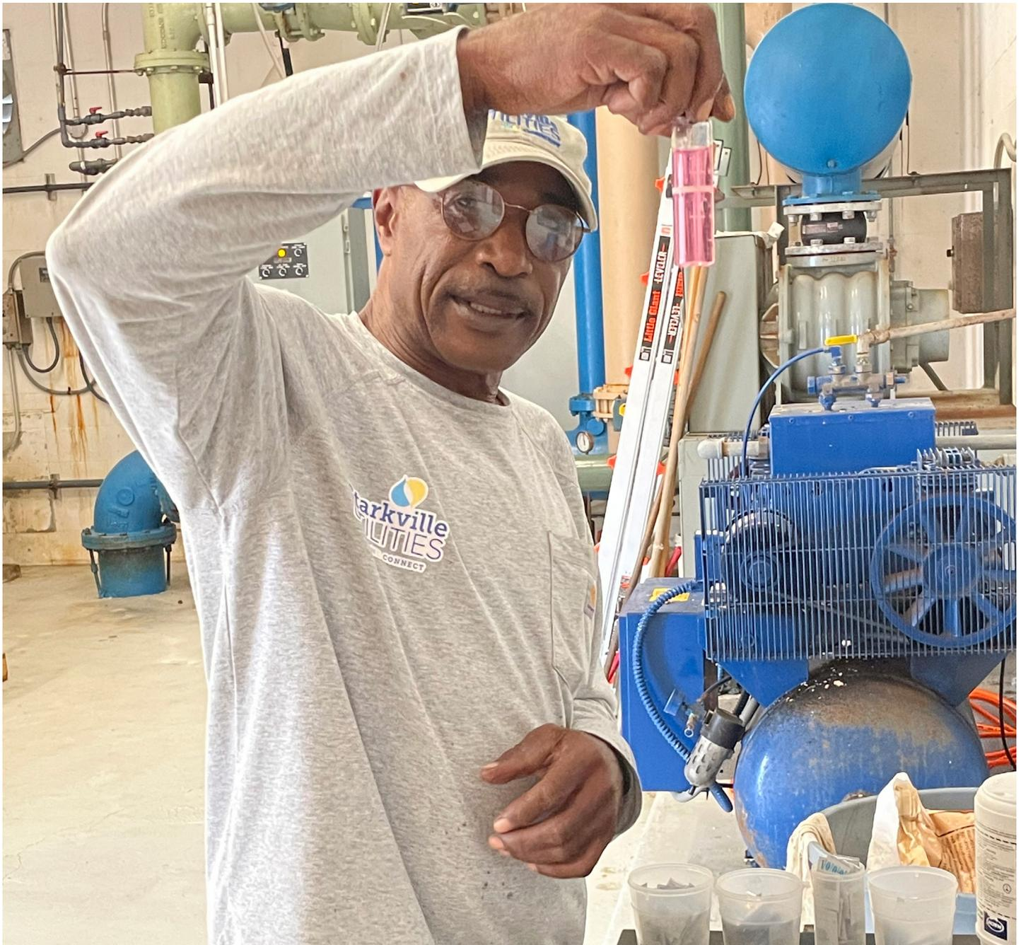
Theodis Weaver, a class C operator with the city of Starkville for 24 years, tests water samples for free residual chlorine at the Starkville Curry Street treatment plant.
