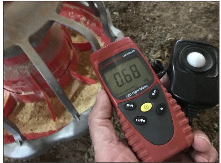
Figure 2. Light level at feed pan (0.68 foot candles) in a broiler house.
