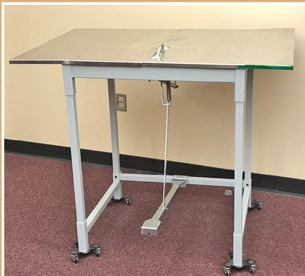
A pedal-operated clamp mechanism attached to a work table is a best practice for commercial producers.
