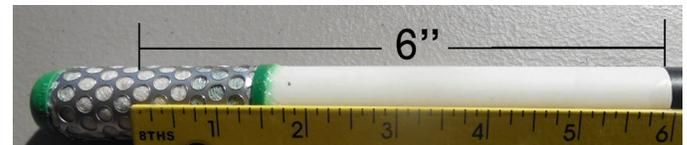
**Step 8:** Slide a rubber cap onto the top end of the PVC section. The construction is now complete!
