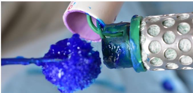
**Step 6:** While aligning the sensor weep slot with the drilled weep hole, push the sensor collar fully into the bottom end of the PVC section.
