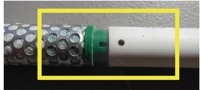
**Step 7:** Wrap a ring of black electrical tape so that the distance between the bottom of the tape and the middle of the attached sensor equals the intended sensor depth. After installation, the bottom edge of the black electrical tape should be flush with the ground.
