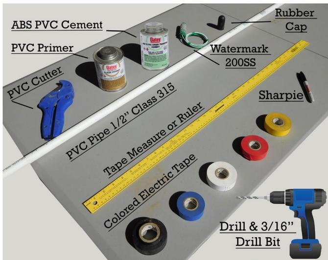
One set of 6-inch, 12-inch, 24-inch, and 36-inch sensors will require one 10-foot stick of 1/2-inch Class 315 PVC pipe. Select the correct PVC specifications to avoid frustrations later.
