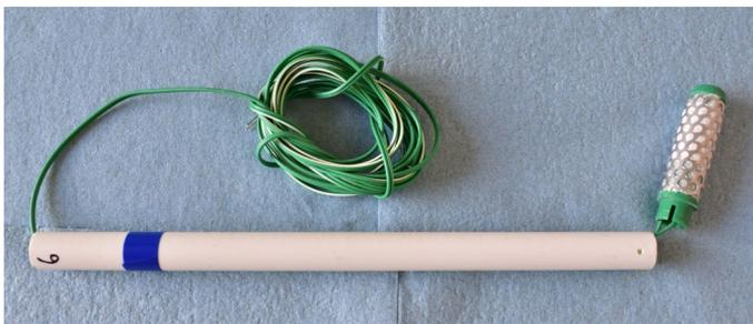
**Step 5:** Carefully apply an appropriate amount of ABS-PVC transition cement to the sensor collar.
