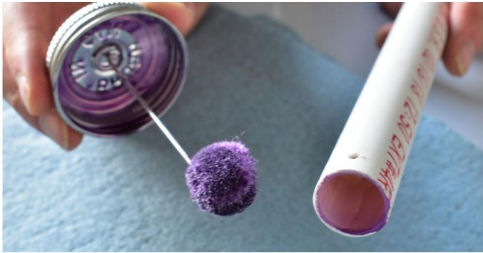
**Step 4:** After a few minutes of drying, thread the sensor wires from the bottom end of the PVC section to the top end until the sensor collar meets the bottom end. Bundle the extra wire.
