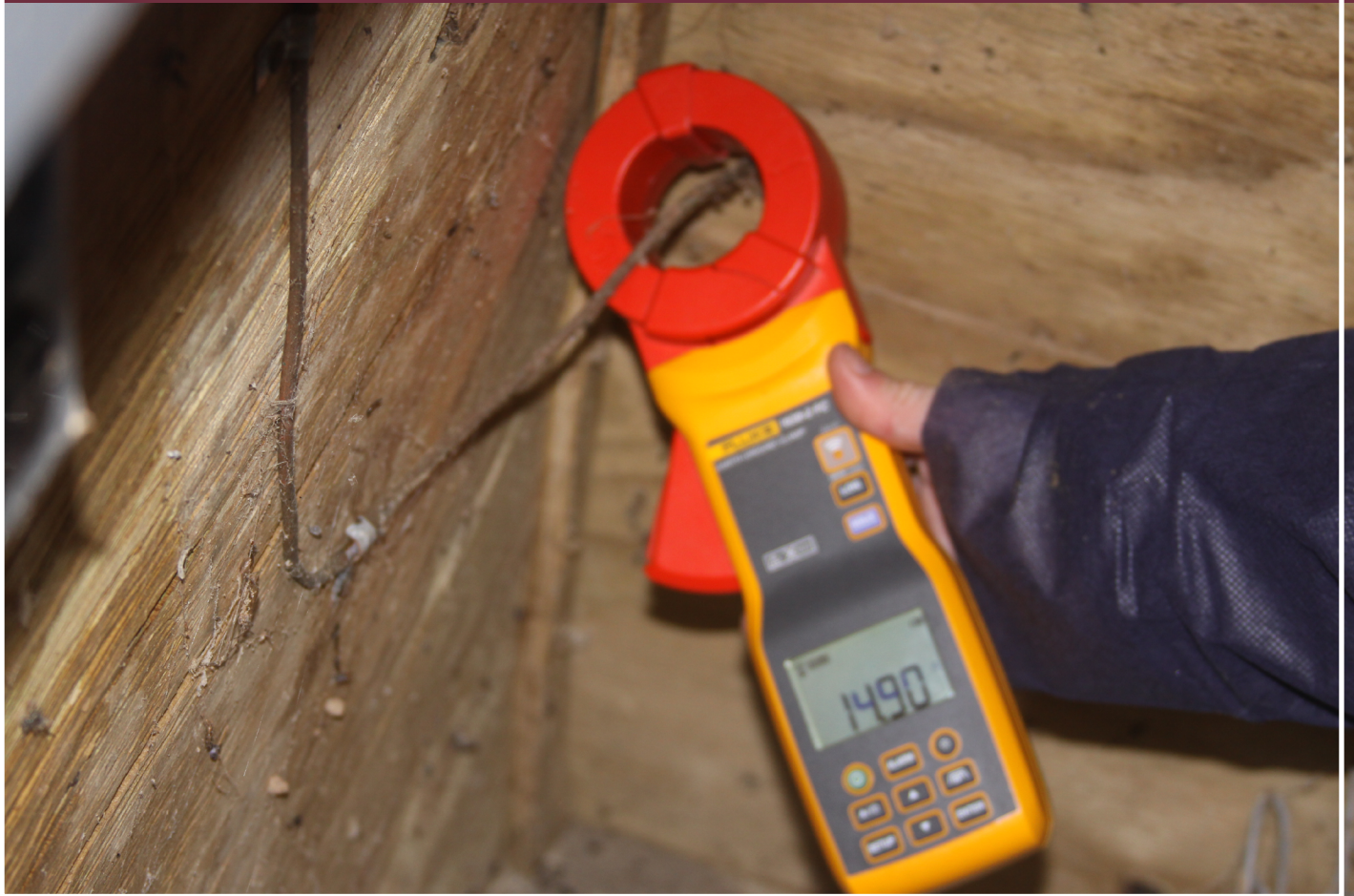
Figure 1. According to the National Electrical Code, a properly grounded system should have an earth ground resistance of 25 ohms ( \Omega ) or less. This properly grounded control room breaker box is reading 14.90 \Omega on the ground resistance meter.
