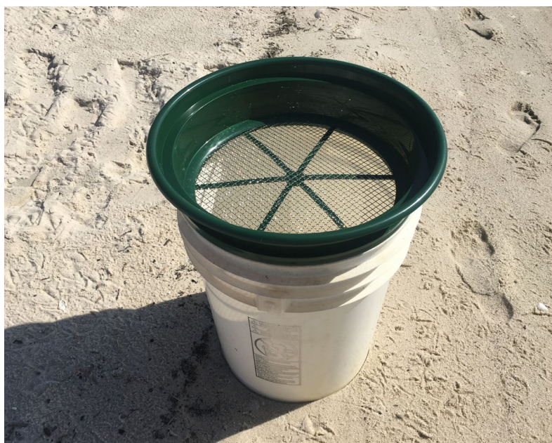
Figure 9. Sieve and bucket used to separate microplastics from sand.
