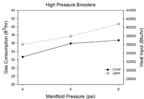
**Figure 3.** Effect of varying manifold pressure on gas consumption and heat input of low- and high-pressure round radiant brooders. The middle point in each line graph represents the rated manifold pressure for the respective brooder.
