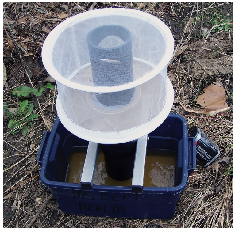
Figure 5. Gravid trap used to trap Culex species.
