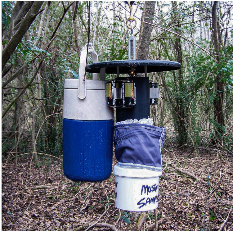
Figure 4. CDC light trap with dry ice as a carbon dioxide source.
