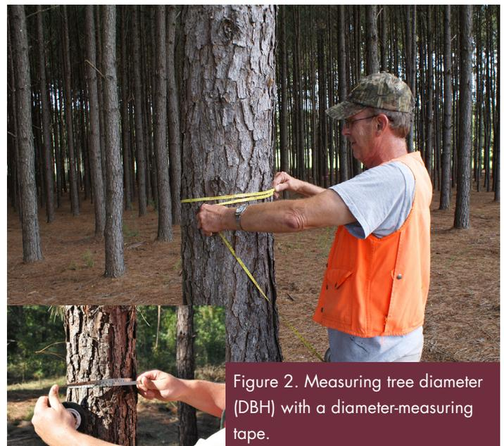
Figure 2. Measuring tree diameter (DBH) with a diameter-measuring tape.
