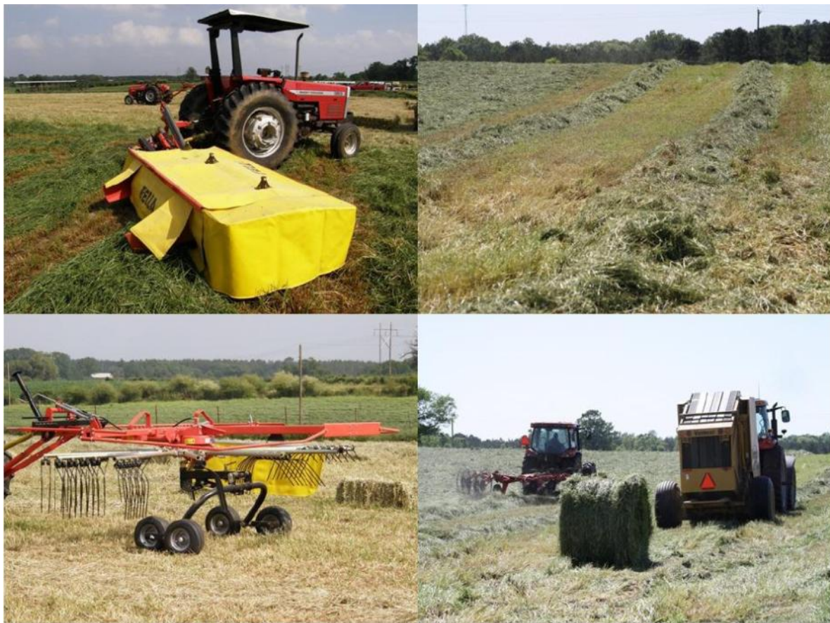
Figure 2. The hay harvesting processes: cutting, tedding, raking, and baling.
