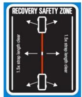
zone of both helpers & watchers before the actual pull begins. If you are operating a winch, position yourself in a safe position such as inside the cab or behind the door. If repositioning is needed, in the middle of a recovery, always loosen tension on the pull line before entering the danger zone.
