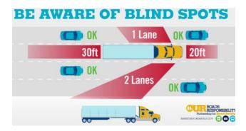
To help avoid blind spots, your vehicle's mirrors must be adjusted correctly. Mirrors are to be adjusted to see the surrounding vehicles, not the back and down the side of your own vehicle. The cabin's center rearview mirror is used to keep an eye on what is coming up from behind, while the outside mirrors reflect the area outside the view of the inside rearview mirror.
