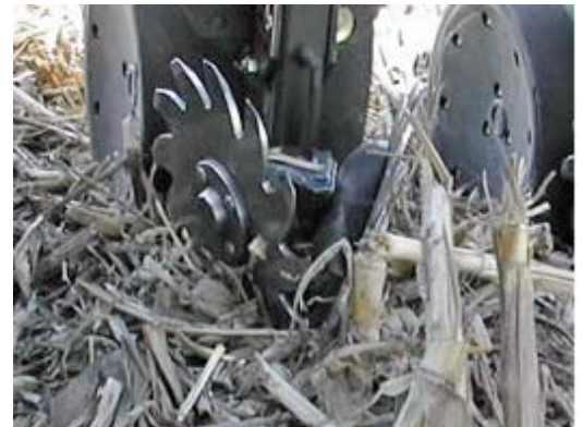
Figure 2. Planter equipped with residue managers to permit planting through heavy corn residue. (Photo courtesy of Yetter Farm Equipment.)
