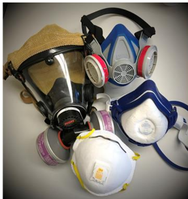
Non-powered APR with Particulate Filtering Elements: clockwise from bottom: disposable N95 FFR; elastomeric full facepiece APR with dual replaceable P100 filters; silicon half facepiece APR with dual replaceable P100 filters; half facepiece APR with replaceable N95 filter (photo Rutgers University).
