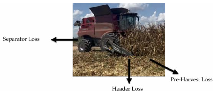
Figure 2. Location of harvest losses on a combine harvester.
