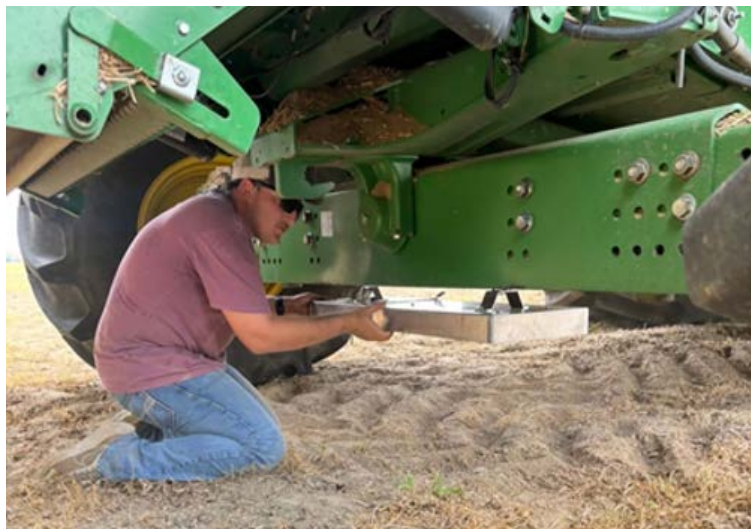
Figure 4. The top image is the drop pan in the field after being dropped from the combine. The bottom image shows the mounting process of the drop pan on the axle of the combine.
