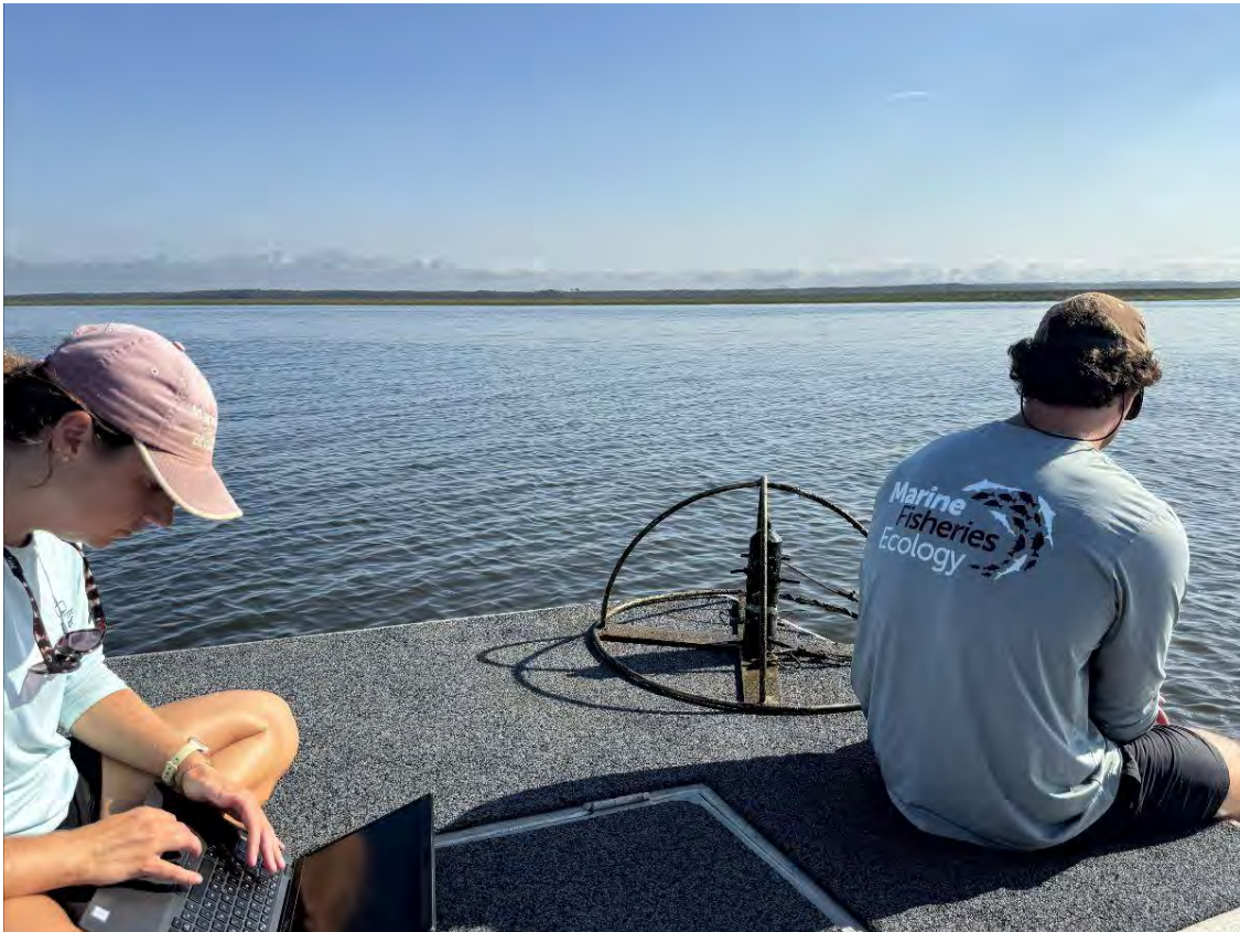
Alena Anderson and Conrad Pfalzgraf download detection data from an acoustic receiver in Grand Bay National Estuarine Research Reserve as part of routine receiver maintenance and data collection.
