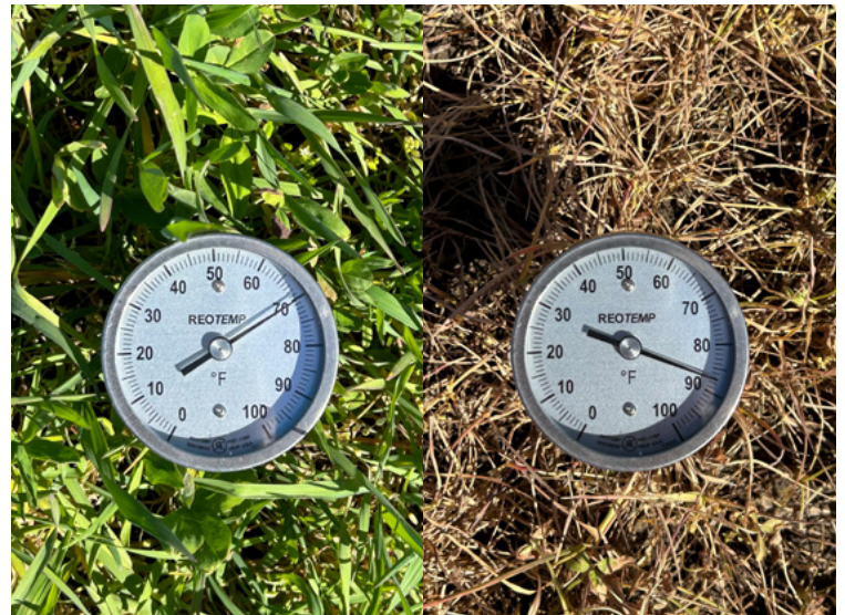
Figure 3. Herbicide timing dramatically affects the soil seedbed environment in cover crop systems. Early termination (as shown on the right) allowed the sunlight to warm the soil and promote subsequent crop growth and higher yield.
