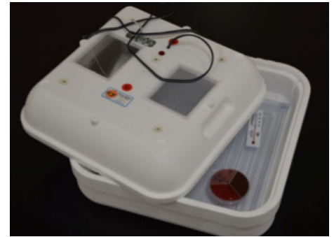
Figure 6. Place the lid back on the tri-plate and place it upside-down in the egg incubator for 24 hours. Turning the plate upside down (so that the agar is on top and the lid is on bottom) will help prevent condensation from flooding the agar, which can prevent bacterial growth.
