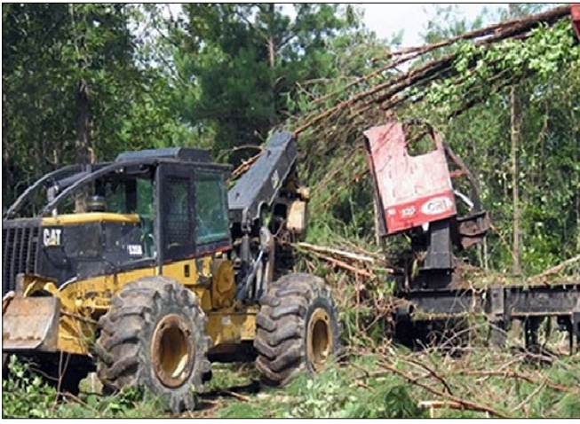
Figure 5. Skidder distributing slash from a loading deck into a thinned pine stand. Photo by James Floyd.
