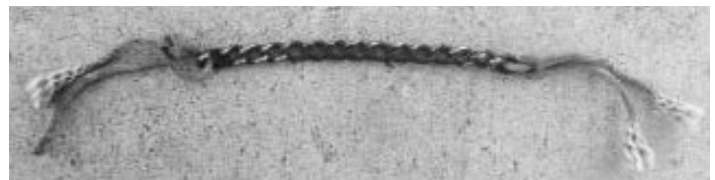
Unacceptable curb chain strap
