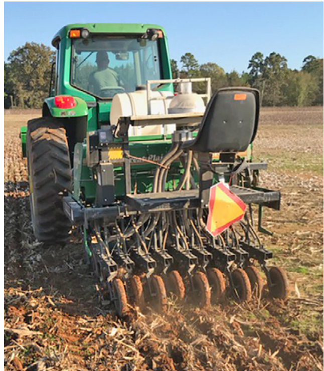
Figure 3. A seed drill allows planting at the proper depth and row spacing and maintains a uniform seeding rate per acre. Photo by Mark Shankle.
