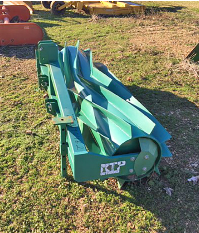
Figure 4. A roller-crimper uses weight to roll down plants, and the chevron pattern crimps the stems to terminate the plant. Water can be added to increase the weight and improve effectiveness.
