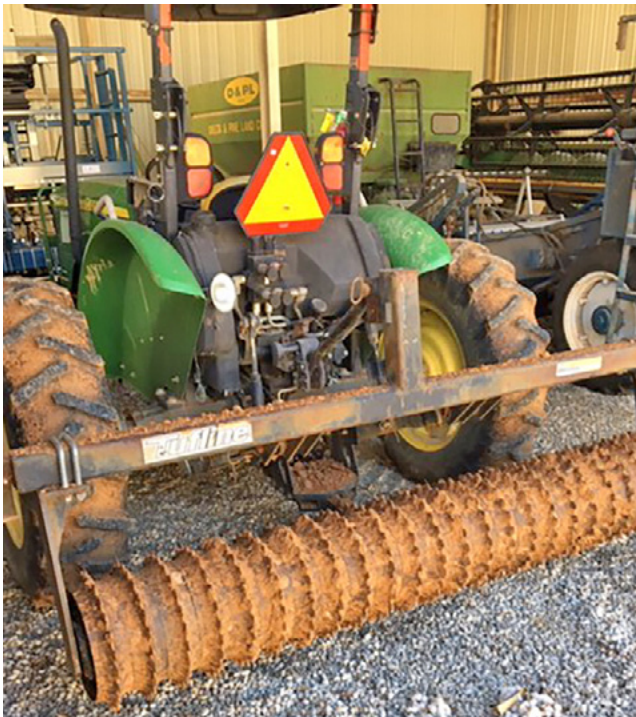
Figure 2. A cultipacker is recommended when broadcast seeding. It provides better seed-to-soil contact and firms the soil to keep new seedling roots from drying out.
