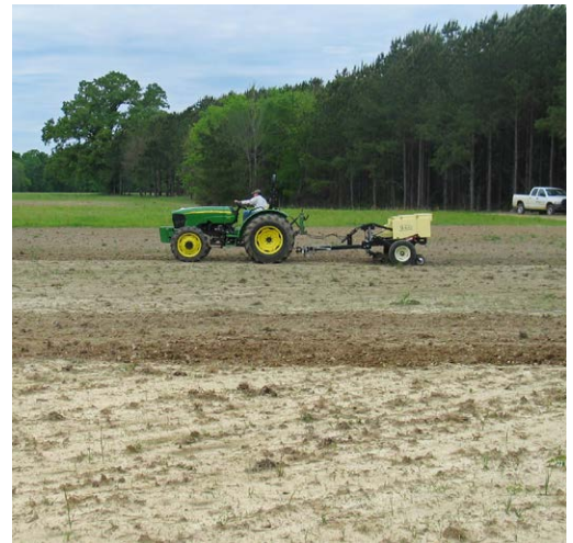
A native warm-season grass seed drill is specially designed to handle these seeds.
