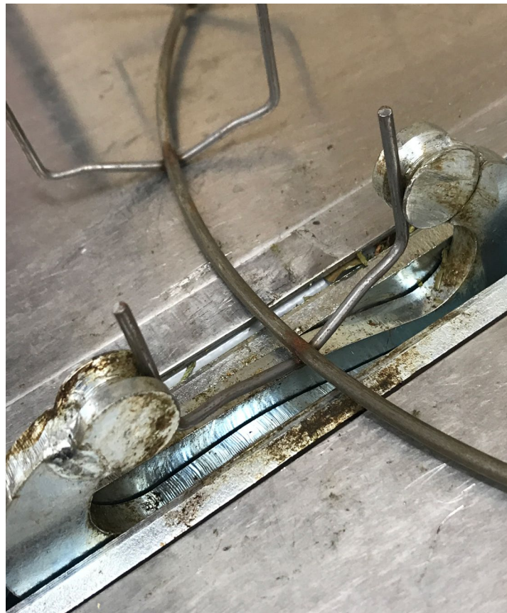
Figure 2. The clamp mechanism pinches heavy-gauge wreath wires around a gathered bunch of plant material stems.
