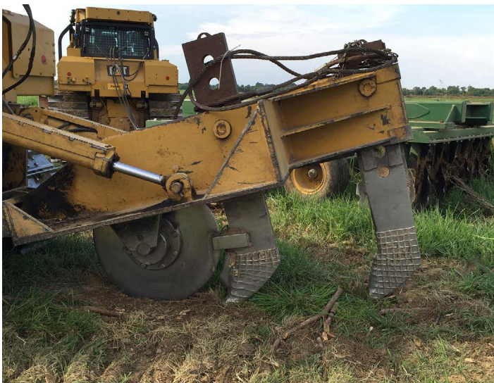
Figures 14 and 15. Offset double-shank subsoil system often used in cutovers. Note heavy-duty construction for increased shear-stress on tracts with increased roots and stumps.
