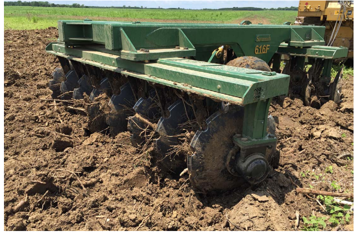
Figure 8. Site preparation disking before planting trees.
