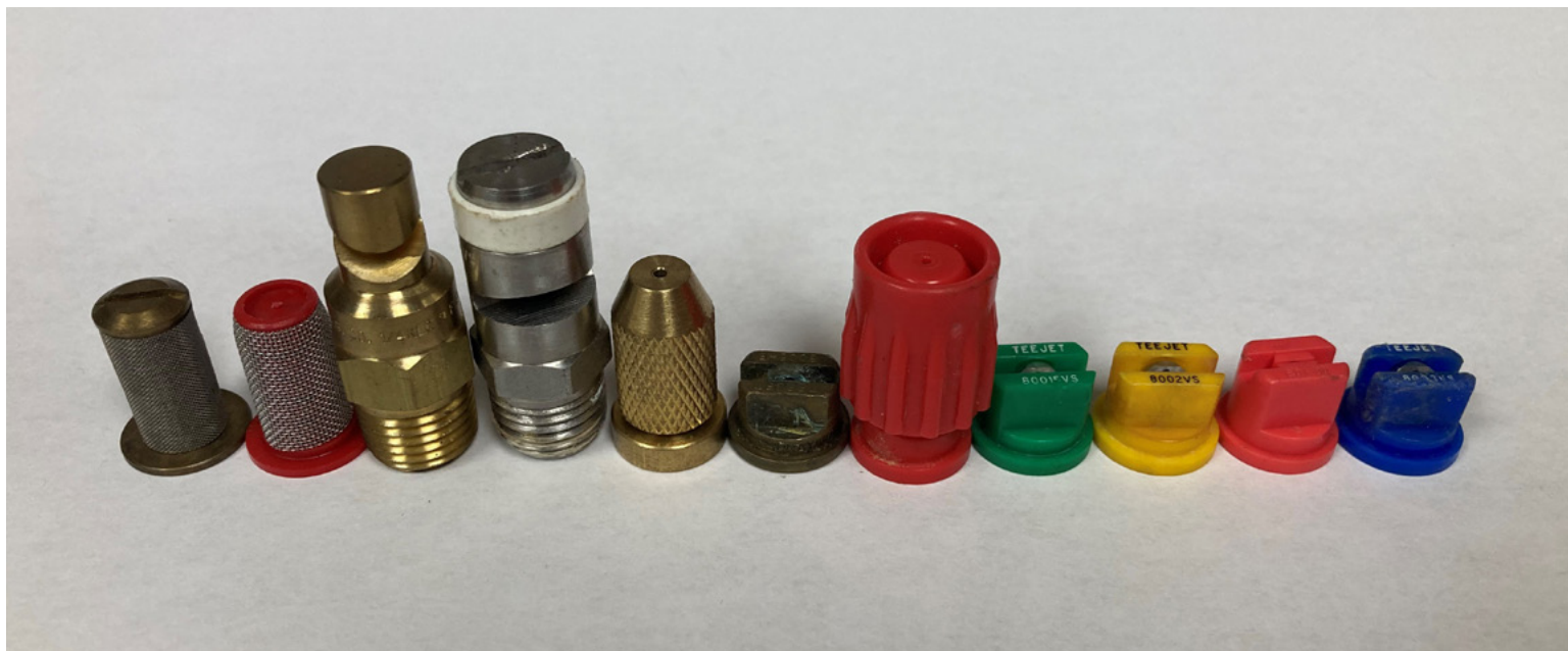
Figure 1. Equipment to be used in applications must be the same as that used in calibration. Identical backpack sprayer models using the same tank pressure may have completely different spray output if different spray nozzles are used. Each of these spray tips and strainers result in different spray output when all other factors are constant.
