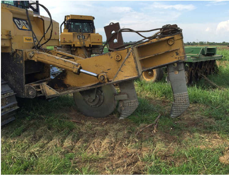
Figure 13. Double shank subsoiler used to prepare a former pasture for planting.
