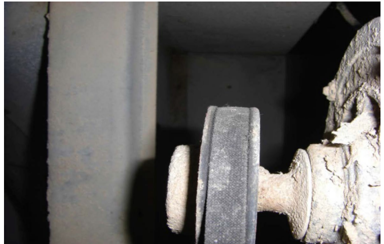
Figure 1. Acceptable belt and pulley wear. Belts should be flush with the outer edge of the pulley or slightly above.
