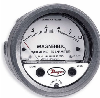
Figure 1. An analog Magnehelic gauge (left) and a digital manometer used to test static pressure.
