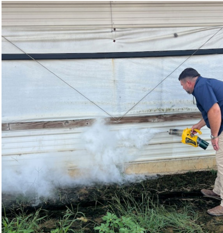
Figure 2. Smoke testing a curtain-sided house to identify air leaks.
