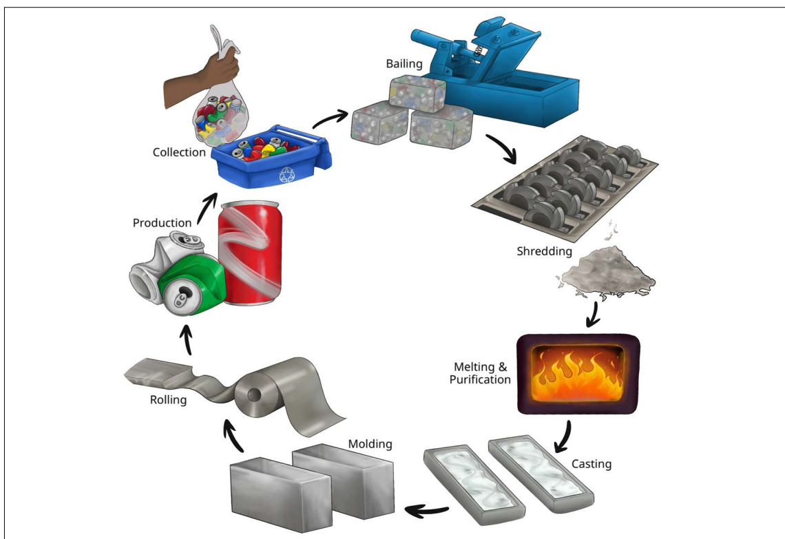
Figure 1. Aluminum can recycling: From scrap to finished cans. Illustrated by Chaisee Bell, Delta Research and Extension Center
